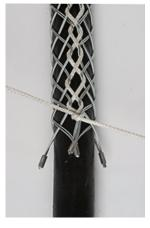
4 Wrap the remaining lace tightly around the end of the grip and secure with an overhand knot. This provides added security from accidental release.
