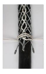
6 Always tape down the mouth of the grip with PVC or similar heavy duty tape to provide a smooth transition from grip to cable.
