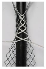
1 Position the grip in the desired location on the cable and begin lacing from the lead or anchoring end of the grip (the end with the eye). Thread the lace through the first two loops and pull through until the lace is centred at this point.
